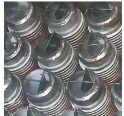
Individual Tube bellows independent differential expansion
